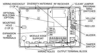
Figure 3B. MCR-308T with Cover Removed
