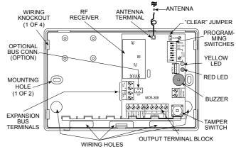
Figure 3A. MCR-308 with Cover Removed
