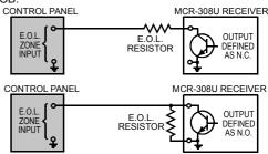
Figure 6. Wiring E.O.L. Zones
