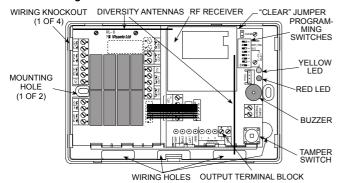
Figure 3C. MCR-308TRL with Cover Removed
