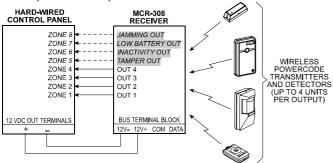
Figure 1. Typical Application of the MCR-308
