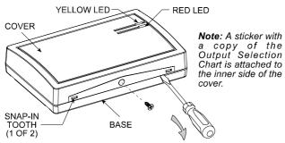
Figure 4. Removing the Top Cover
