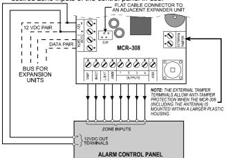
Figure 5. Wiring Diagram
