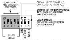
Figure 7. DIP Switch Tasks and Positions
